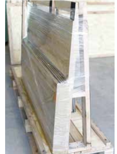
The ideal storage of CORSTONE for a longer period should be on easels with an angle 6° of the base in relation to the backrest and the backrest must have several crossbars for ensure the full support of the boards.
